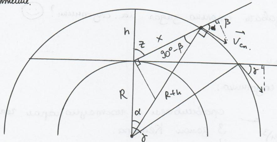
$$\beta = 90^\circ - (180^\circ - \alpha - (180^\circ - z)) = 90^\circ - (z - \alpha) = 90^\circ + \alpha - z$$
